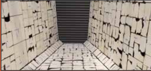
Grip Tight - a superior bond achieved between ceramics and steel for increased wear life
